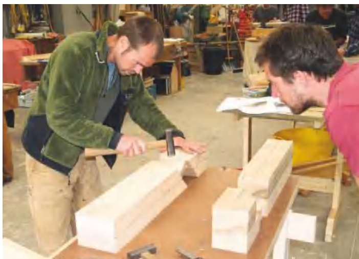
▲ Pic.13 Killing the fibres. Just hammer the surface where the joint fits, insert the joint, and the natural moisture in the air will expand the fibres again for a really solid fit
